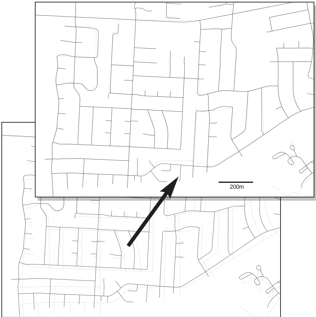
Figure 3. VITAL's rubber-streeting algorithm applies a geometric adjustment to an erroneous map to make it agree with a more accurately surveyed map or datum. Useful attributes associated with the geometrically poor map are retained, or easily transferred to the other map.
