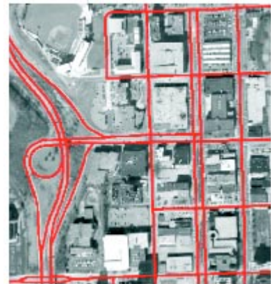
Figure 1. Road network extracted from six-inch, high-resolution imagery.
