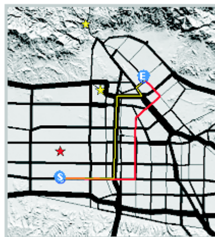
Figure 3. REDARS adjusted least cost route (red line) in response to bridge collapse. The original route is shown in yellow.
