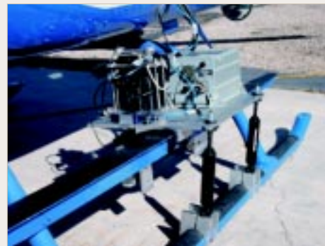
Figure 2. DGPS and IMU unit mounted on helicopter.
