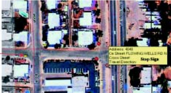
Large scale photography used for inventory of street signage. The yellow triangles are yield signs; the red circles are stop signs. Credit: Pima
