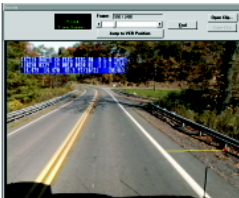
Distance from guard-rail post to edge of pavement is measured in Roadware's Surveyor module. Courtesy: Roadware, www.roadware.com
