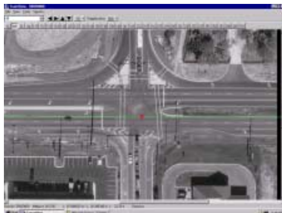
Centerline and intersection identified on aerial photography, for linear measurement. Credit: Florida DOT
